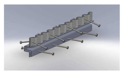
The HC-Omega Sinus Slide® construction and expansion joint has a body which is made of two continuous cold-rolled profiles in 5 mm thick SJ235JRG2 steel.
