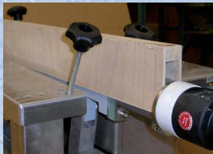
*In the cooled state the wood protection has to be attached. After lowering the heater blade the machine is in basic position*
